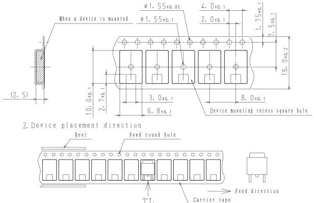
TL Carrier tapeThose with one electrode terminal on the feed hole side.....TL
