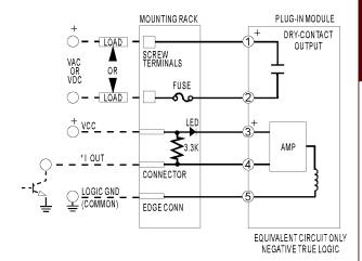
\* Control line is compatible with totem pole or tri-state output device.
