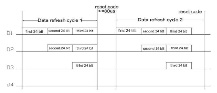
Note: The data of D1 is send by MCU, and D2, D3, D4 through pixel internal reshaping amplification to transmit.
