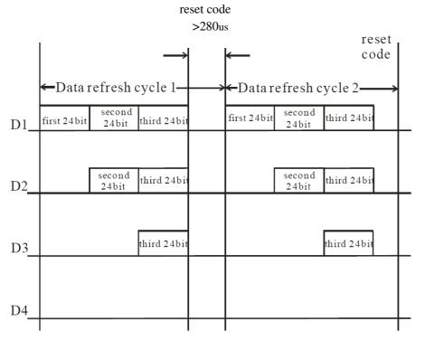
Note: The data of D1 is send by MCU, and D2, D3, D4 through pixel internal reshaping amplification to transmit.
