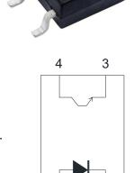
1 Anode 2 Cathode 3 Emitter 4 Collector
