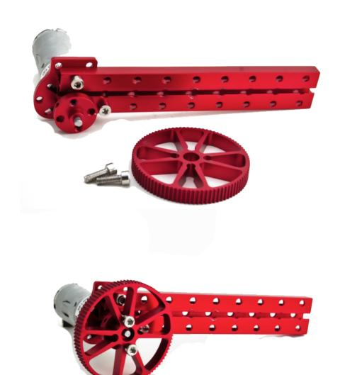
Attach the Rim to the motor bracket with the M4 screws.
