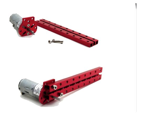
Attach the mounted DC motor to the **Double Beam 09** with the **M4 screws**.
