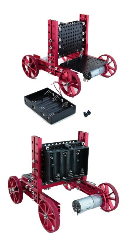
Attach the **battery pack** to the Triangular Tank with the **rivets**.
