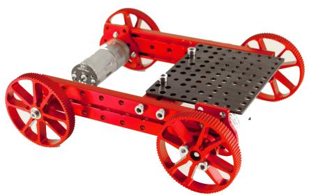
Attach the **base plate** with the **M4\*14 screws** to the assembled wheel frame. secure with **M4 nuts.**
