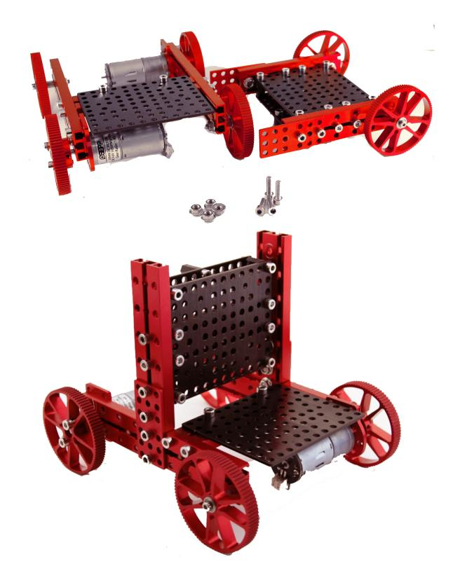
Attach the entire top bracket to the bottom RIM bracket with **M4\*14 screws**. Fasten with the **M4 nuts**.
