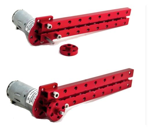
Place the **plastic ring** first through the DC motor shaft. Attach the shaft connector to the DC motor shaft. Tighten the headless screw.
