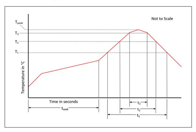
Figure 8: Solder Reflow Profile
