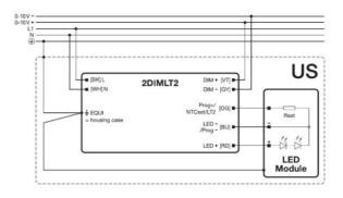
494748\_Wiring Diagramm 2DIMLT2 with NTC
