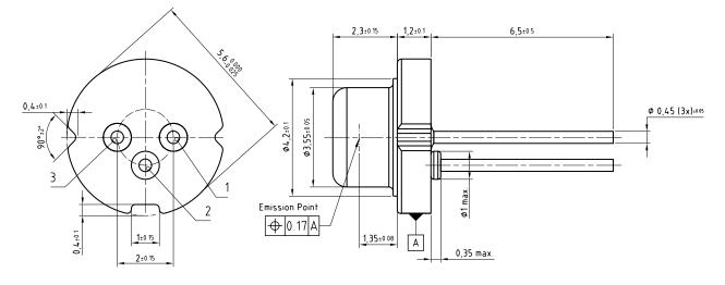
Pin 1: LD Anode Pin 2: LD Cathode, PD Anode (case) Pin 3: PD Cathode
