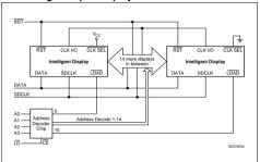
Multiple displays can be cascaded using the CLKSEL and CLK I/O pins (Figure ,Cascading Multiple Display"). The display designated as the MasterClock source should have its CLKSEL pin tied high and the slaves should have their CLKSEL pins tied low. All CLK I/O pins should be tied together. One display CLK I/O can drive 15 slave CLK I/Os. Use RST to synchronize all display counters.
