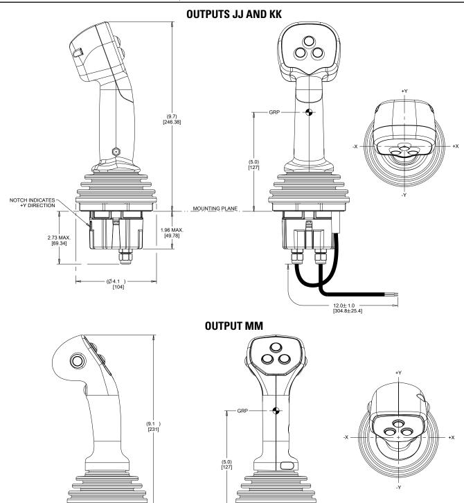
Wires and strain relief not shown in all views for clarity.
