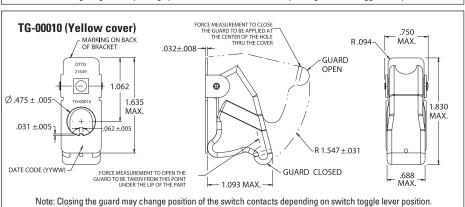
Note: Opening or closing the guard shall not change position of the switch contacts.
