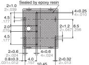
Dimension: Tolerance Max. 1mm .039 inch: ±0.1 ±.004 1 to 3mm .039 to .118 inch: ±0.2 ±.008 Min. 3mm .118 inch:  $\pm 0.3 \pm .012$
