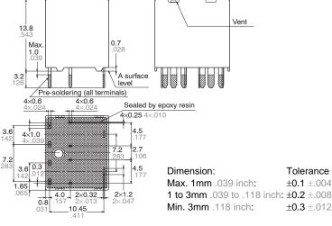
Dimensions (thickness and width) of terminal is measured before pre-soldering. Intervals between terminals is measured at A surface level.
