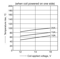
1.-(3) Coil temperature rise (at room temperature)
