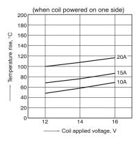
1.-(5) Coil temperature rise (at room temperature)
