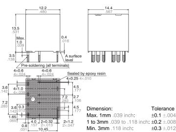
Dimensions (thickness and width) of terminal is measured before pre-soldering.
