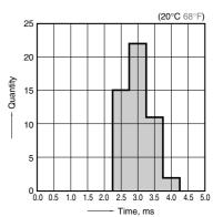
6. Functional shock resistance Tested sample: AEJ11012, 3 pcs. Half-wave pulse of sine wave: 11 ms Detection time: 10μs. Applied direction: 6 directions Applied cycle: Each of 3 cycles
