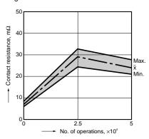
5-(2). Electrical life test (5 A 250 V AC, resistive load) Sample: ALA2PF12, 6 pcs. Operation frequency: 20 times/min. (ON/OFF = 1.5s: 1.5s) Ambient temperature: 20°C 68°F
