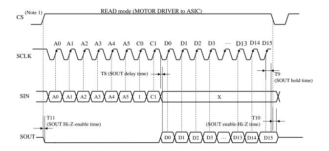
Note 1) CS default value of each cycle (Write / Read mode) starts from Low-level. Note 2) It is necessary to input the system clock OSCIN at write mode.
