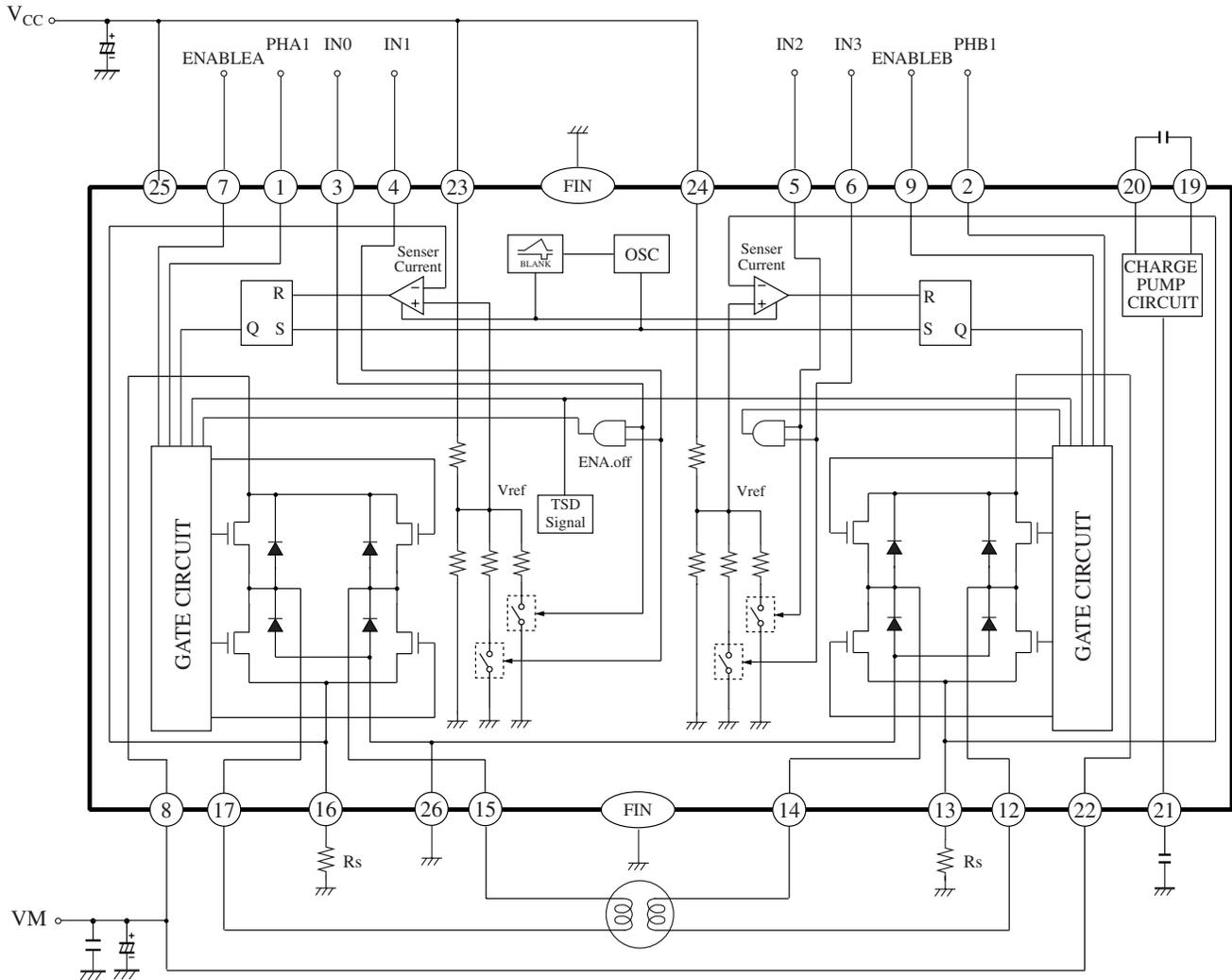
\* A voltage is applied externally to Terminals PHA1, PHB1, IN0 to 3, ENABLEA, ENABLEB, VREFA and VREFV, and may cause an overcurrent. To protect the device from overcurrent, insert an overcurrent protective resistor (1K $\Omega$  or over).
