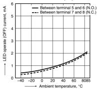
6. LED reverse current vs. ambient temperature characteristics Load voltage: 400 V (DC);
