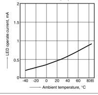
6. LED turn off current vs. ambient temperature characteristics Load voltage: Max. (DC)
