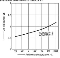
2.-(2) On resistance vs. ambient temperature characteristics
