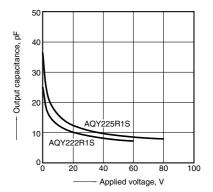
12.-(2) Output capacitance vs. applied voltage characteristics Measured portion: between terminals 3 and 4
