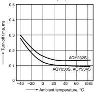
temperature characteristics Sample: All types; Load voltage: Max. (DC); Continuous load current: Max. (DC)
