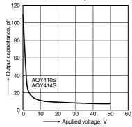
12-(2). Output capacitance vs. applied voltage characteristics
