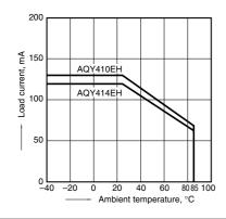
1-(2). Load current vs. ambient temperature characteristics
