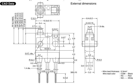
■ Wire leads right side type: Mounting hole 3 mm, standard type
