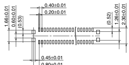
Recommended metal mask pattern Metal mask thickness: When 120μm (Terminal opening ratio: 70%) (Metal-part opening ratio: 100%)
