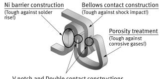
V notch and Double contact constructions (Tough against exposure to foreign particles and solder flux!)
