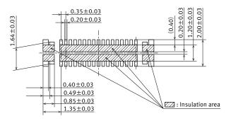
Recommended metal mask pattern Metal mask thickness: When 100 μm (Terminal opening ratio: 70%)
