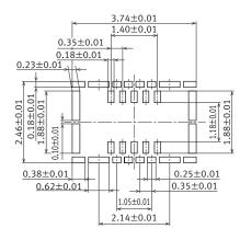
Recommended metal mask pattern Metal mask thickness: When 80 µm (Signal terminal opening ratio: 74%) (Ground terminal opening ratio: 70%)
