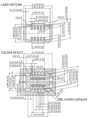
Recommended metal mask pattern Metal mask thickness: When 80 µm (Signal terminal opening ratio: 80%) (Ground terminal opening ratio: 90%)
