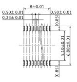
Keep the PC board warp no more than 0.03 mm in relation to the overall length of the connector.
