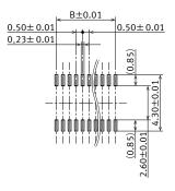
Recommended metal mask pattern Metal mask thickness: When 120 µm (Opening area ratio: 69%)
