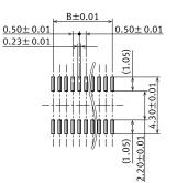
Note : See the dimension table for more information on the B dimension of the socket and header.
