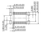
Recommended metal mask pattern Metal mask thickness: When 150 µm (Terminal opening ratio: 48%) (Metal-part opening ratio: 100%)
