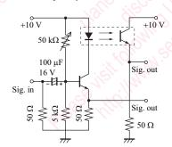
Measurement circuit of frequency characteristics
