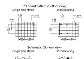
Note: External dimensions of 1 coil latching types are same as single side stable type.
