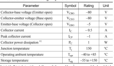
Note) \*1: Printed circuit board: Copper foil area of 1 cm<sup>2</sup> or more, and the board thickness of 1.7 mm for the collector portion Absolute maximum rating without heat sink for P<sub>C</sub> is 0.5 W
