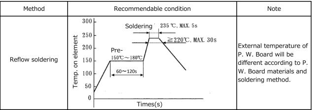
\* When performing reflow soldering, an appropriate coating thickness of cream solder is 0.10 mm to 0.15 mm.
