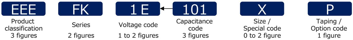
◇ FK, TG, EB series with  $\phi D \geq 12.5\text{mm}$
