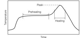
• Recommended soldering conditions for flow
