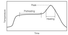
Recommended soldering conditions for flow
