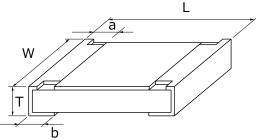
Unit: mm **Dimensions** Mass (Weight) Part No. W (g/1000 pcs) ERJU2R 1.00±0.05  $0.50 \pm 0.05$  $0.20\pm0.10$  $0.25 \pm 0.10$  $0.35 \pm 0.05$ 0.8 ERJU3R 0.80+0.15/-0.05 0.45±0.10  $1.60\pm0.15$  $0.30\pm0.20$  $0.30 \pm 0.15$ 2 ERJU6R 2.00±0.20 1.25±0.10 0.40±0.20 0.40±0.20 0.60±0.10 4
