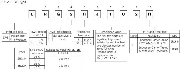
The above example 2 shows a metal oxide film resistor SMD type, 2 W power rating, resistance value of 1.0 kΩ, tolerance ±5 %,and embossed taping.
