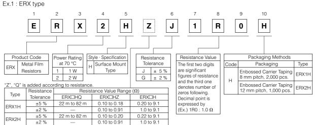
The above example 1 shows a metal film resistor SMD type, 2 W power rating, resistance value of 1.0 Ω, tolerance ±5 %, and embossed taping.
