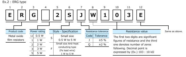
The above example 2 shows a small metal oxide film resistor, 2 W power rating, resistance value of 10 k $\Omega$ , tolerance  $\pm 5$  %, and package of radial taping.
