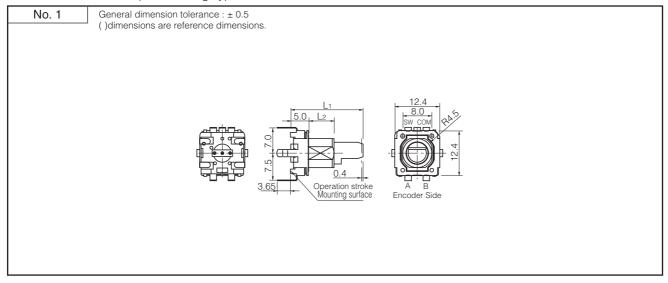
• Standard rotation-torque / Bushing Type with Sleeve / with Switches .......With detents : EVEJBE
