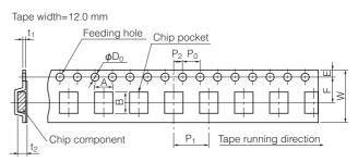
Taping condition: Lack of products in the middle of taping should be one MAX, but total quantity specified in the specifications should be secured.
