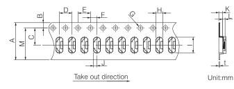
Taping condition: Lack of products in the middle of taping should be one MAX, but total quantity specified in the specifications should be secured. Peeling off strength of top tape: It should be within 0.2N to 1.0N at 165 degree in peeling off angle.
