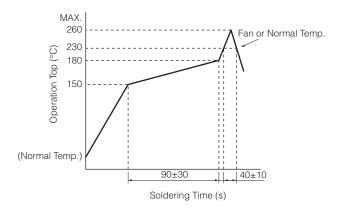
\* Reflow temperature may vary by location even in the same reflow condition. Please check the reflow temperature at terminals and at the top of a switch to make sure the both temperatures are withiin the specification. If even one of them is out of the specifi cations, please adjust.
