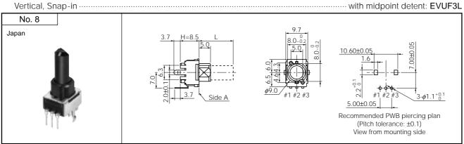
• Shaft Trims and Dimensions in mm for Type without Bushing (Drawings are at full CCW position.) Type F (Flat)
