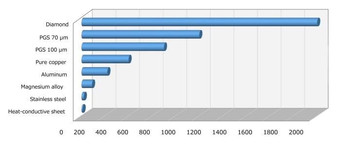
Coefficient of thermal conductivity W/(m·K)
