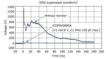
\*IEC61000-4-2 ··· International Standard of the ESD testing method (HBM) for electronic equipment ability to withstand ESD generated from a human body. It sets 4 levels of severity
