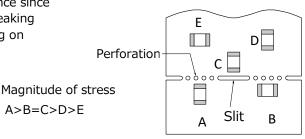
(3) The magnitude of mechanical stress applied to the Varistors when dividing the circuit board in descending order is as follows: push back < slit < V-groove < perforation. Also take into account the layout of the Varistors and the dividing/breaking method.
