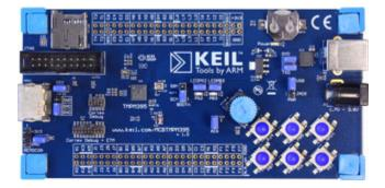
The Keil MCBTMPM395 Evaluation Boards enable you to create and test working programs based on the Toshiba TMPM395 family of ARM Cortex<sup>™</sup>-M3 processor-based devices.
