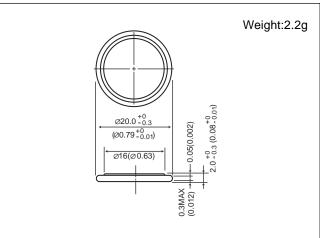
**Note:** This bare cell diagram is for size reference only. Please refer to the tab configurations at the end of this section for available tabs.
