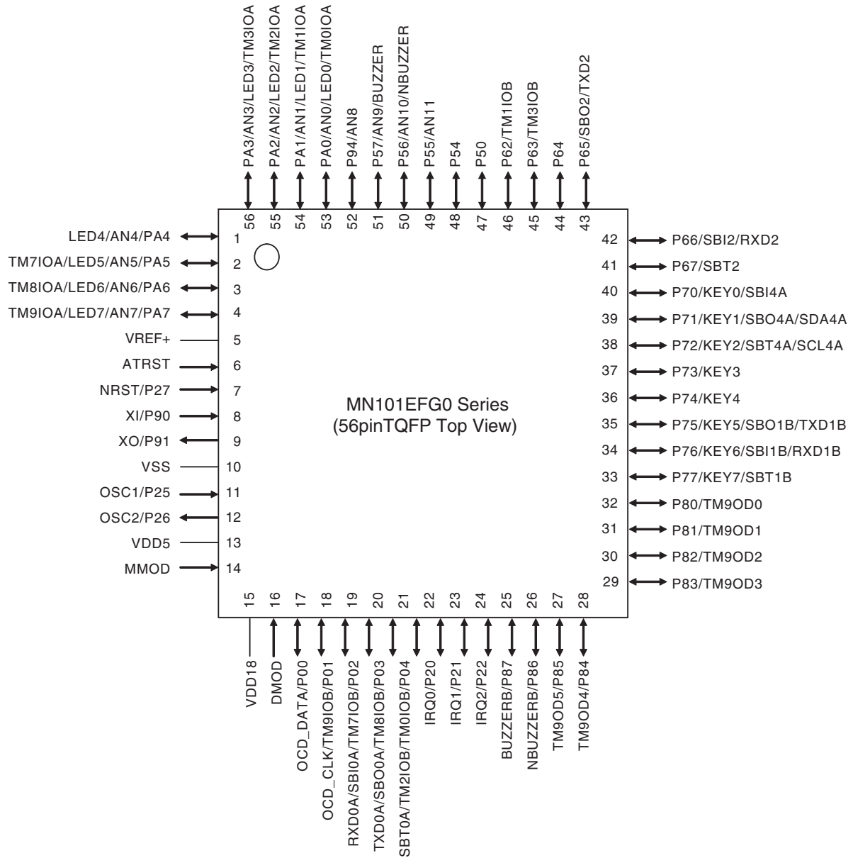
Figure:1.3.5 Pin Configuration (MN101EFG0 Series 56-pin TQFP)
