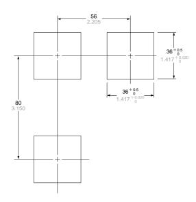
Note: The panel thickness should be 1 to 3.2 mm  $0.039\ to\ 0.126\ in.$
