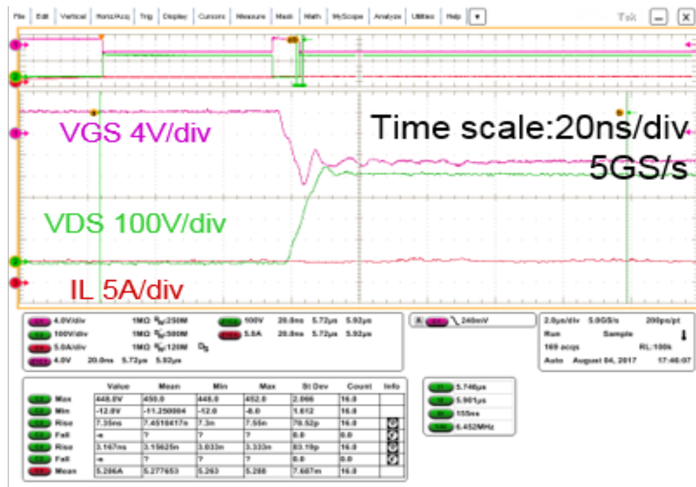
Figure 16(b): Typical turn-off waveform
