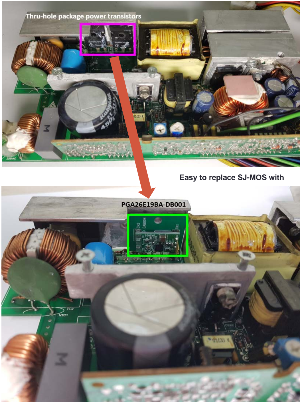
Figure 12: For illustration purpose, PGA26E19BA-DB001 is conveniently mounted on an actual power supply
